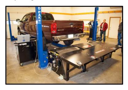
J&J Performance is a chassis dynamometer, tuning, and performance shop built around a Dynocom 15,000 Series Chassis Dynamometer. This state-of-the-art equipment is capable of handling up to 15,000 ft-lbs of torque, 2,400+HP, and 240+ MPH. That should be enough capability for any of our Injectors' car, eh? J&J offers custom tuning with the best engine/ECM tuning available.
